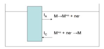
(i) If the equilibrium cell reaction is  $Mn^{n+} = Mn + ne^{-}$  and the cathodic and anodic current are as indicated in the Figure above, define exchange current density and write an expression (in terms of current for the exchange current density (3 marks)
