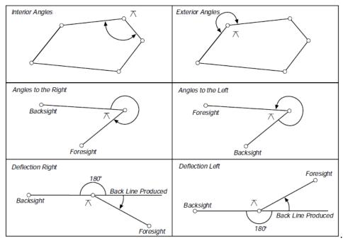
Figure 12: Types of Angle Measurements.
