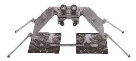
Figure 18; Mirror Stereoscopic viewer
