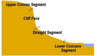
Fig.ure 8 Show the element of slope
