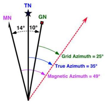
Figure 4. Declination difference between Grid, True, and Magnetic North.
