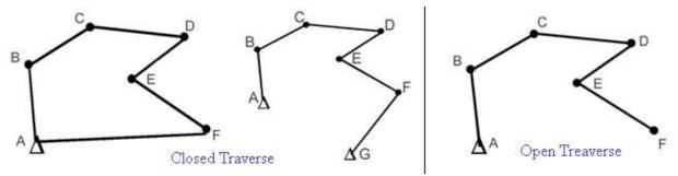
Figure 13: Examples of survey traverses.
