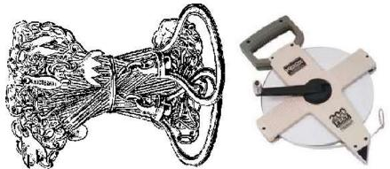
Figure 11: Gunter's chain and measuring tape.
