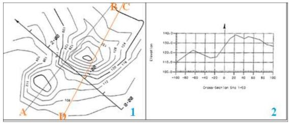
Figure 32 Terrain cross section cutting.
