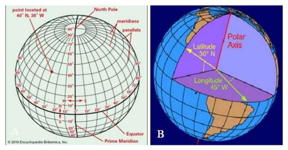
Figure 1a, b: Measurement of latitude and longitude relative to the equator, the Prime Meridian and the Earth's rotational or polar axis.
