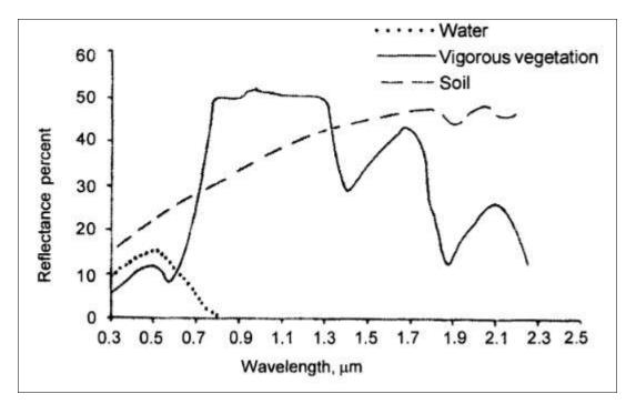
Figure 22. Spectral Signatures of Typical Features of earth's Surface.
