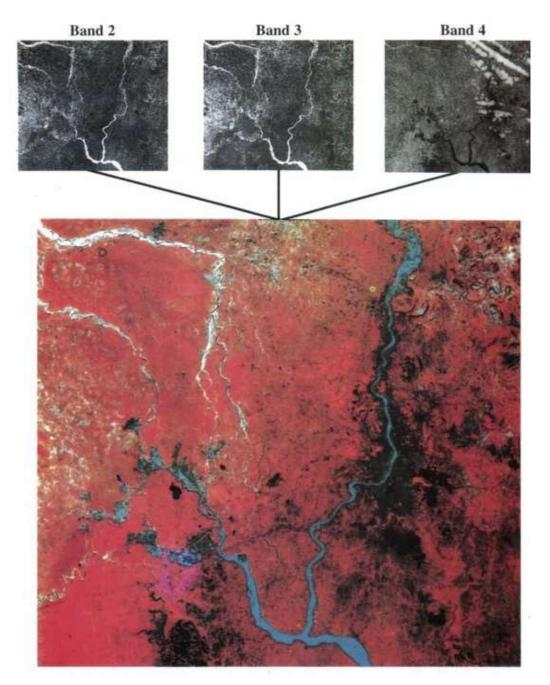
Figure 25:I RS- 1 0 LISS-11i FCC image (bands 2, 3, 4) and corresponding Black and White Images of band 2, band 3 and band 4 data of path .108, row 56, showing Calcutta and Surrounding Areas.
