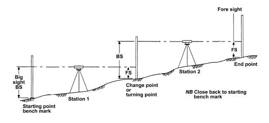
Figure 16. Method of traverse levelling.
