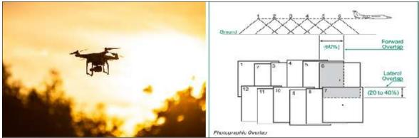
Figure 17: Photo flight line and overlaps
