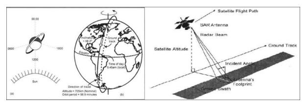
Figure 20; Sun synchronous orbiting satellite.
