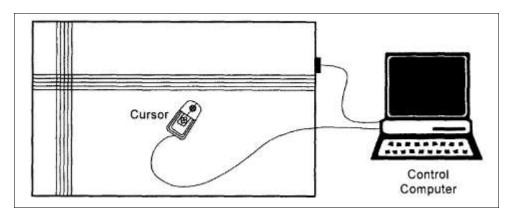
Figure 27 Contemporary wires embedded tablets digitizer. To achieve good results, the following steps are necessary.
