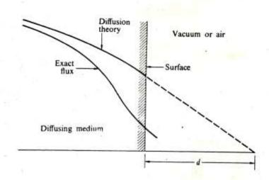
Fig.1.2: The Extrapolation Distance at a Surface
