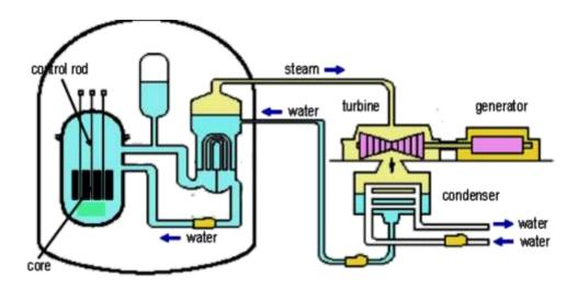
Fig.1.6: Pressurised-Water Reactor (PWR)
