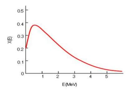
Fig. 1.2: Fission Neutron Energy Spectrum
