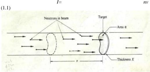
Fig.1.1: Neutron Beam Striking a Target
