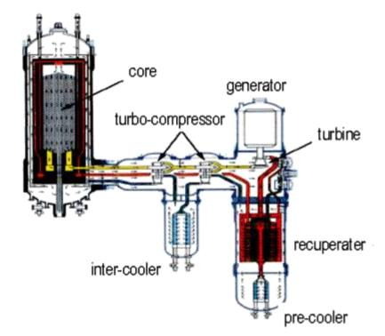
Fig. 1.7: High-Temperature Gas-Cooled Reactor
