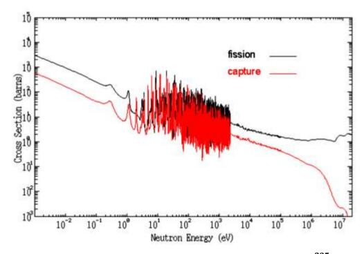
Fig. 1.1: Fission and Capture Cross Sections for  $^{235}U$
