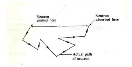
Fig.1.3: Trajectory of a Neutron in Moderating Medium
