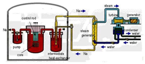
Fig. 1.8: Fast Breeder Reactor (Loop-Type)
