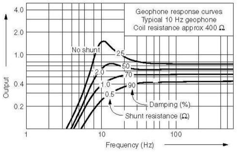
Fig. 3.2: Frequency Response of a Typical Moving-coil Geophone
