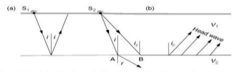
Fig. 1.2:(a) Reflection and (b) Refraction: Simple RefractionOccurs at A while Critical Refraction Occurs at B
