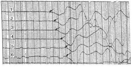
Fig. 4.2: Six-channel Refraction Record Showing Refraction "Picks'
