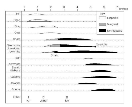
Fig. 1.1: Ranges of P-wave Velocities and Rippabilities in Common Rocks. The Vertical axis, for each Rock type, is intended to show approximately the Relative Numbers of Samples that would show a given Velocity
