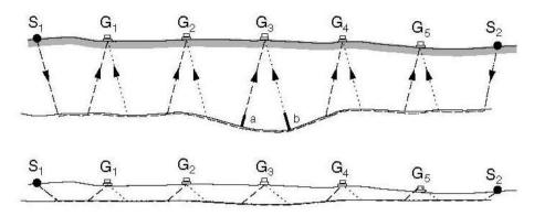
Fig. 2.3: Effect on Travel Times of a Bedrock Depression
