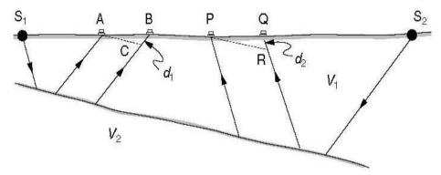
Fig. 2.2: Refraction at a Dipping Interface
