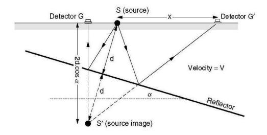
Fig. 1.3: Effect of Dip on a Single-fold Record
