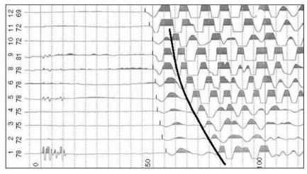
Fig. 1.2: Enhancement Seismograph Record showing Curved Alignment of Reflections (the thick line)
