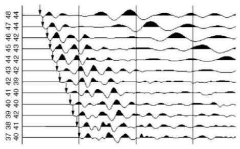
Fig. 1.2: Portion of a Multi-channel Refraction Record, with first-break ""picks" Identified by arrows
