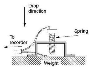
Fig. 2.3: Weight-drop Contact Switch
