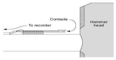
Fig. 2.2: "Post-Office Relay" Impact Switch on the back of a Sledgehammer Handle
