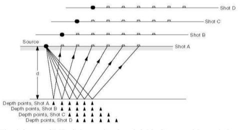
Fig. 2.2: CMP Schematic, for 3-fold Cover with a 6-channel System
