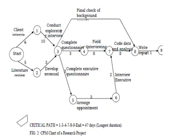
In the CPM chart - above, the nodes represent major milestones and the arrows suggest the work needed to get to each milestone. More than one arrow pointing to a node indicates that all those tasks must be completed before the milestone has been met. A number is usually placed on the arrow "shaft" showing the number of days or weeks required for that task to be completed. Once you have drawn the CPM chart, it draws your attention to two points:
