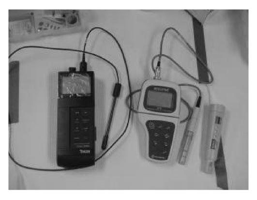
These three meters and probes can measure pH (left) and electrical conductivity (center and right
