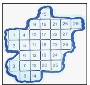
Fig. 3.1: A numbered grid map of an area to be sampled
