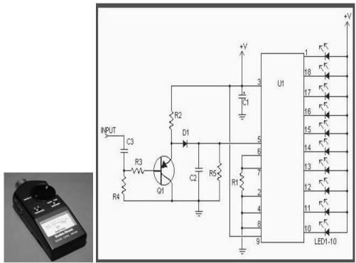
Electric circuit of a sound meter
