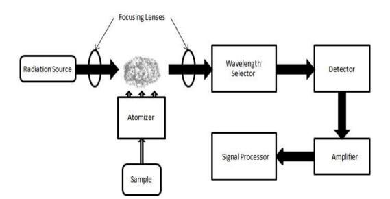
Fig. 5.1: A block diagram of a typical AAS
