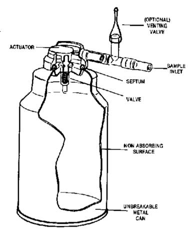
Fig. 6.1: A typical steel evacuated sampler
