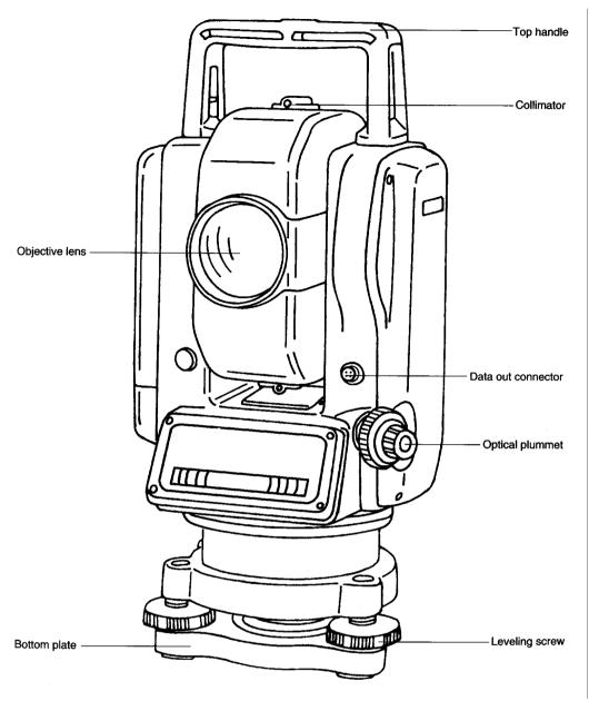
Fig. 2.4: Image of a Total station
