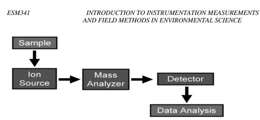
Fig. 5.3: an operational scheme of a Mass Spectrometer
