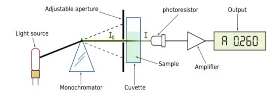
Fig. 5.2: Composition of a typical colorimeter
