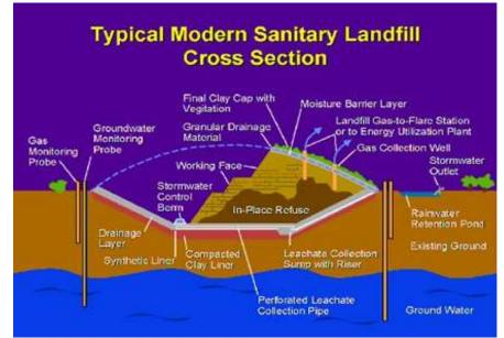
**Fig. 1.2a: Cross Section of a Typical Landfill Operation** Source:<u>http://armypubs.army.mil/eng/DR\_pubs/DR\_a/pdf/tm5\_814\_5.p</u>
