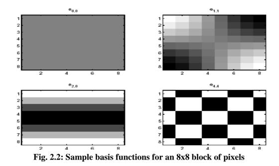
The above four have been chosen out of a possible set of 64 basis functions.
