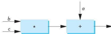
FIGURE 1.1(c) Arithmetic pipeline (Ed Angel (1991))
