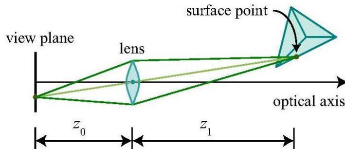
Figure 2.2(a): Thin lens models
