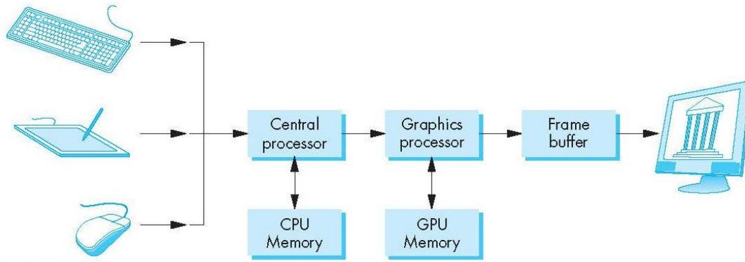
Figure 1.1(a): A graphic system (Engel et al., 1991)
