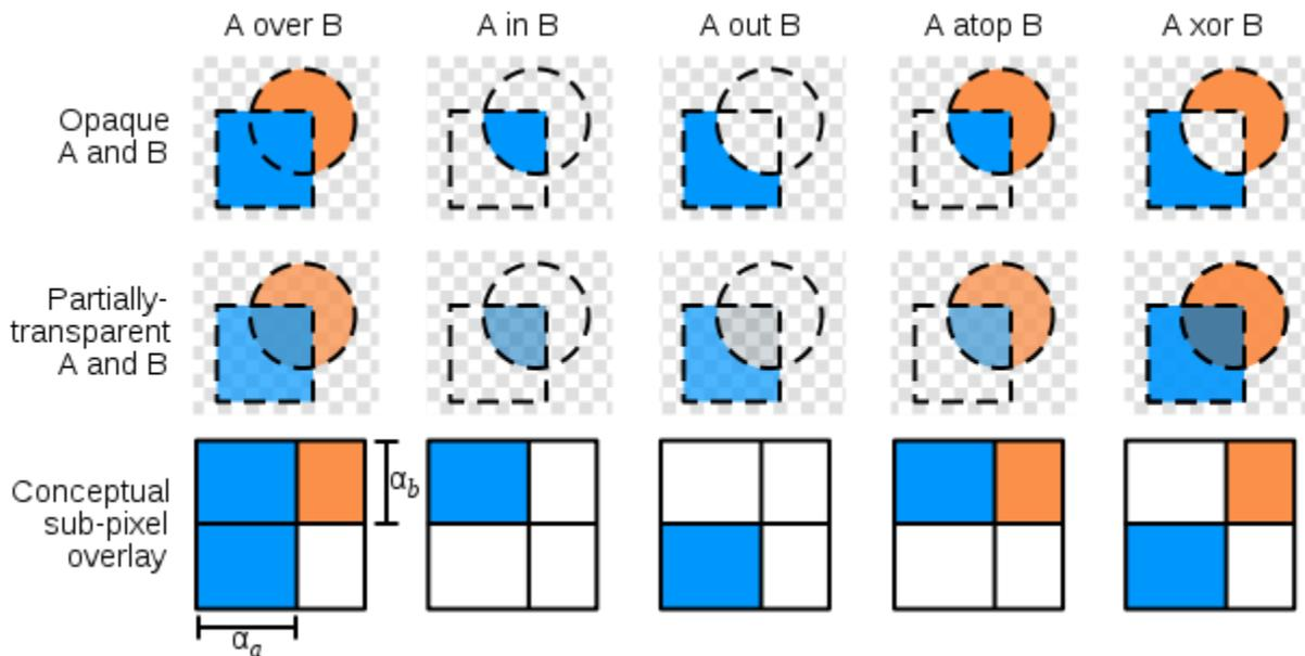
Figure 4.3(a): Alpha compositing of image A and B
