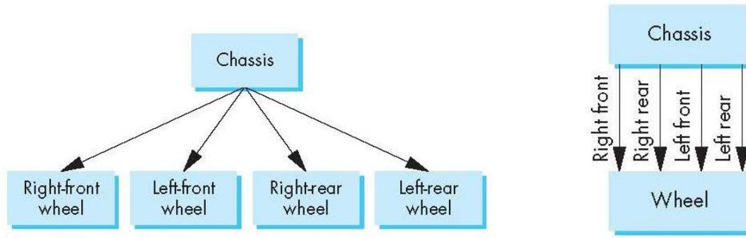
Figure 3.1 (b): Tree structure for an automobile. Fig 3.1(c): DAC model for an automobile (Ed Angel, 1991)
