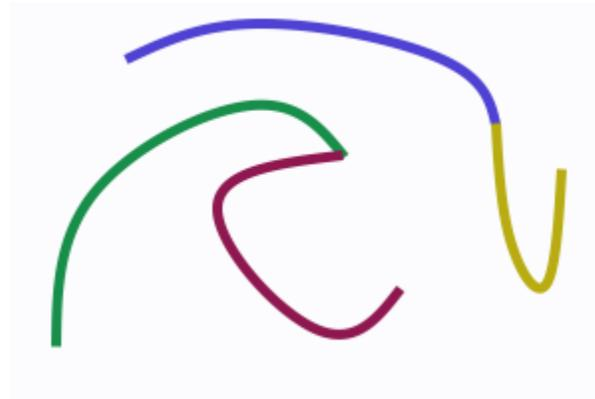
figure 4.1(b): B-Splines consist of Bézier arcs.
