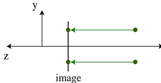
Figure 2.2(g): orthographic projection
