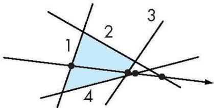
FIGURE 5.1(i) Ray intersecting a convex polygon
