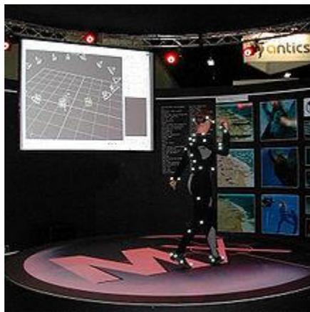
Figure3.3(c): optical motion capture system, Grookda Oger, 2010)
