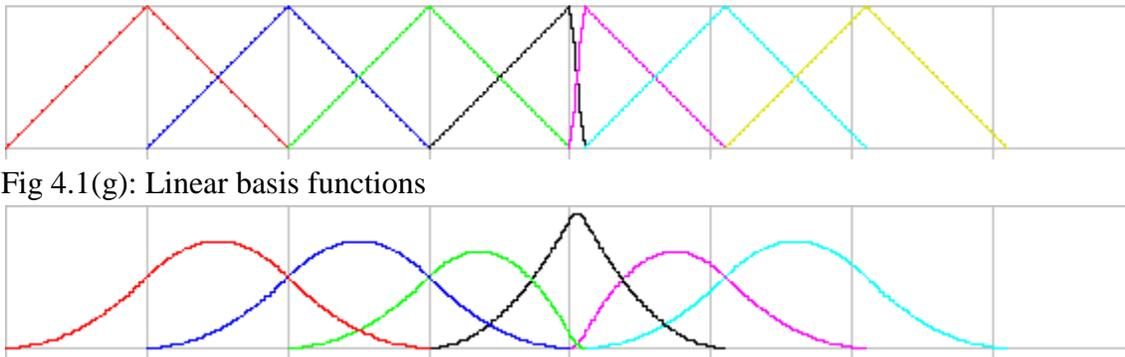
Fig 4.1(g): Linear basis functions
