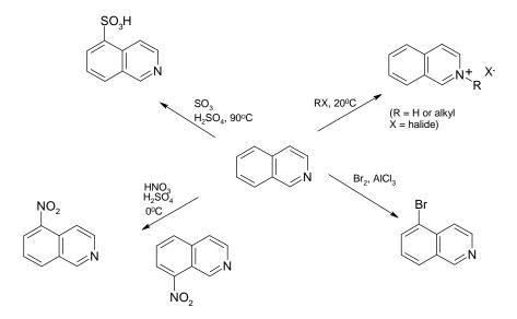
Scheme 15: Reactions of Isoquinolines with Electrophiles
