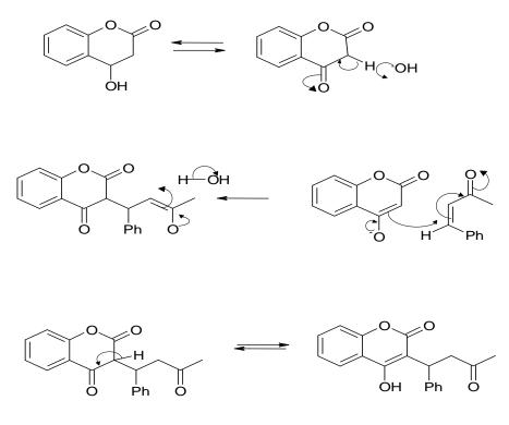
The yield for this synthesis when carried out in water (4-8 h reflux) is typically 40 %. Higher yields can be obtained by carrying out the reaction in methanol (20 h reflux), isolating the product formed and hydrolysing with acid. Typical yields are 93 %.
