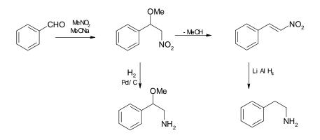
Scheme 18: Synthesis of  $\beta$ -phenylethylamine
