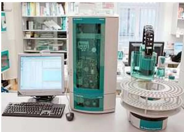
**Figure 3.6** *Metrohm 850 Ion chromatography system*
