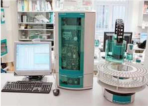
**Figure 3.6** *Metrohm 850 Ion chromatography system*
