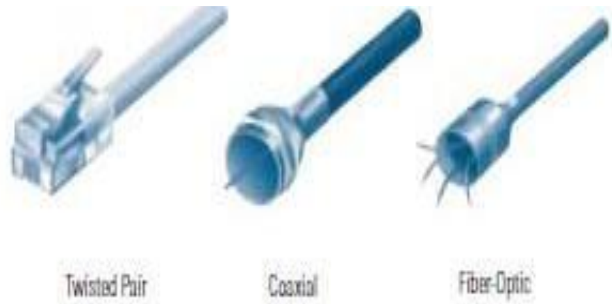
Figure 11.9 The three primary types of Networking cables Source: (Cisco Networking Essentials, 2009).
