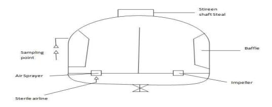
In a fermenter with strict aseptic requirement, it is important to select materials that can withstand repeated steam sterilization. On a small scale, glass stainless steel can be used. Glass gives smooth surfaces; it is not toxic and corrosion-free. It is usually easy to examine the process while it is going on.
