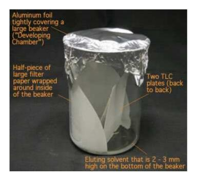
Plate 2.2: Plate Showing TLC Developing Tank
