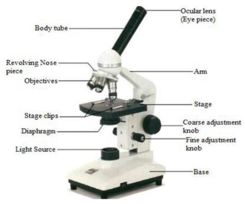
Figure 1.1: Compound Microscope
