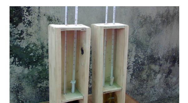
Figure . Locally constructed Hygrometer
