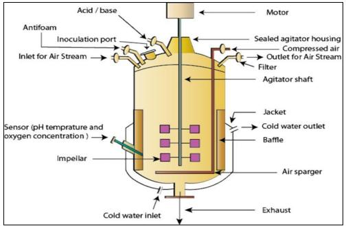
Figure 5.1: Diagram of a typical bioreactor.
