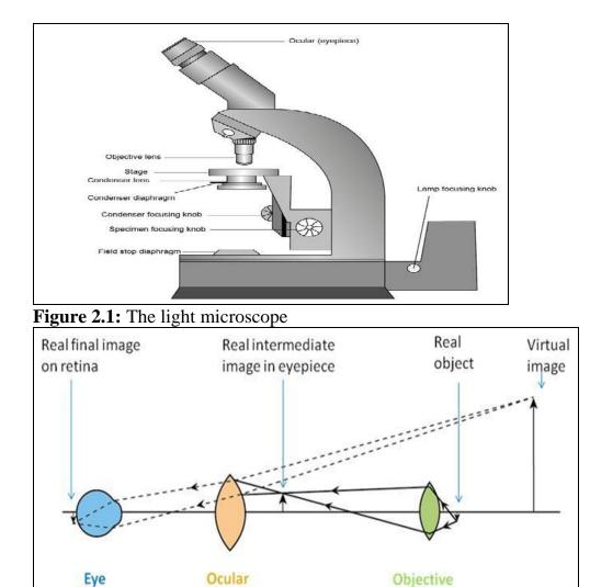
**Figure 2.2:** Perception of a magnified virtual image of a specimen in a microscope
