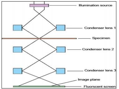
Figure 3.3: Organisation of Transmission Electron Microscope
