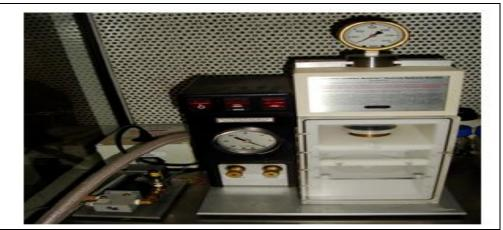
Figure 2.1: A gene gun apparatus
