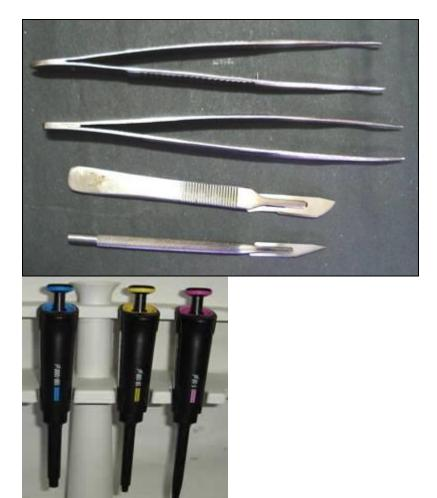
Figure 5.10: a) Forceps and scalpels for dissection and b) Micropipettes.
