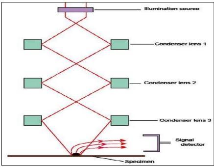
Figure 3.2: Configuration of scanning electron microscope
