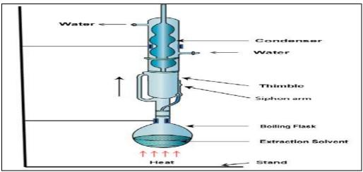
Figure 2.1: A Soxhlet apparatus
