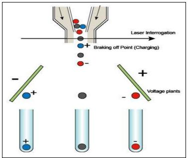
Figure 4.1: Electrostatic flow sorting
