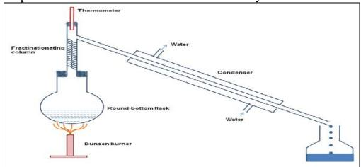
Figure 3.1: A simple fraction distillation apparatus
