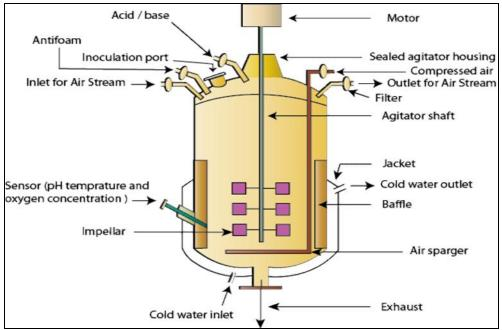
Figure 5.1: Diagram of a typical bioreactor.
