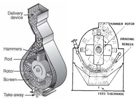
Diagram of a Hammer Mill Machine
