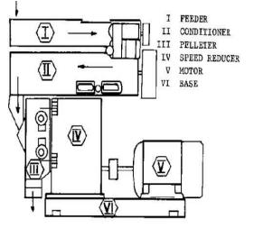
Diagram of Pellet Mill Machines and Parts
