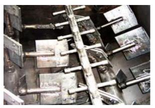
Diagram of a Horizontal Feed Mixer
