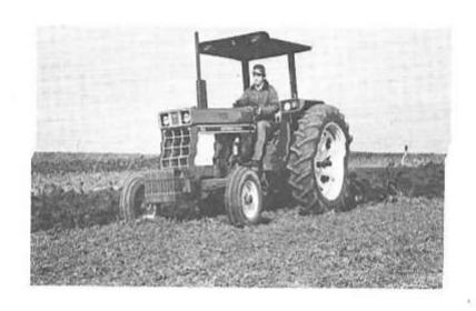
FIG. 16-3. Utility tractor, 65 h.p.; can be used for row crops. (Courtesy International Harvester)
