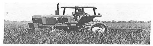
Tractor with extra-high clearance for sugar cane. (Courtesy Deere and
