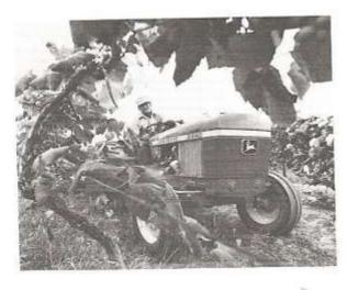
FIG. 16-10. Vineyard tractor, narrow with low profile. (Courtesy Deere and Company)
