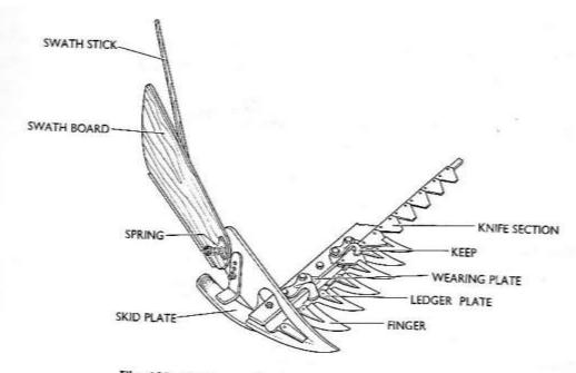
Fig. 122. Cutting mechanism of a mower cutter-bar.
