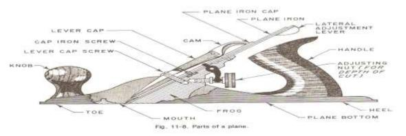
**Plane:** is a fool for shaping disk plow wood using mosle power to force the cutting blade over the wood surface.
