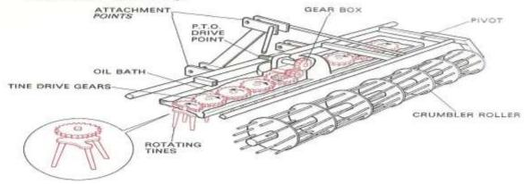
Fig. 104. Working components of a mounted rotary cultivator.
