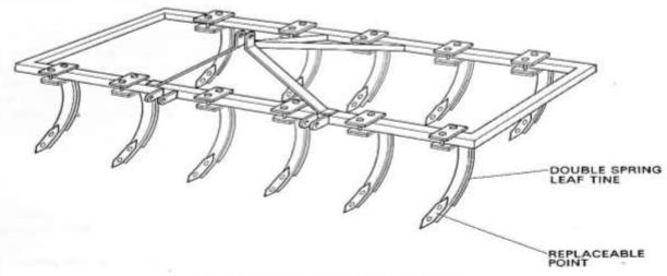
Fig. 98. A mounted spring-tine cultivator.
