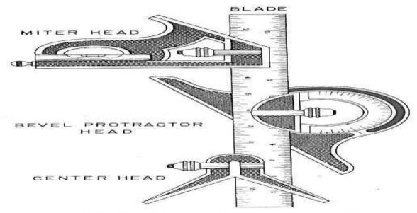
Fig. 6-2. Heads for combination-square blade
