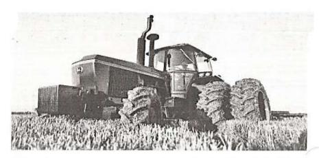
FIG. 16-7. Two-wheel drive tractor with optional front wheel power drive. (Courtes Deere and Company)
