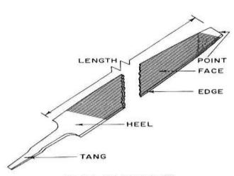
Fig. 6-8. The parts of a file.
