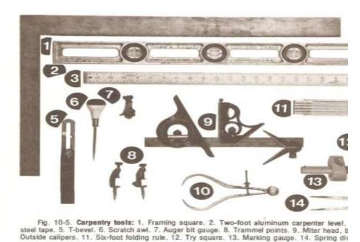
Outside calipers. 11. Six-foot folding rule. 12. Try square. 13. Marking gauge. 14. Spring of
