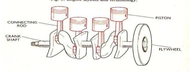
Fig. 6. A four-cylinder engine crankshaft with connecting rods and pistons.
