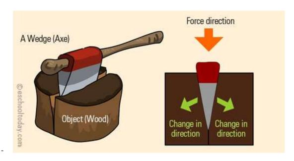
From the above, you will notice that the force applied to the thick end of the wedge overcomes the resistance of the wood. The force is directed downwards, but the wedge directs the force sideways as it drives into the wood.
